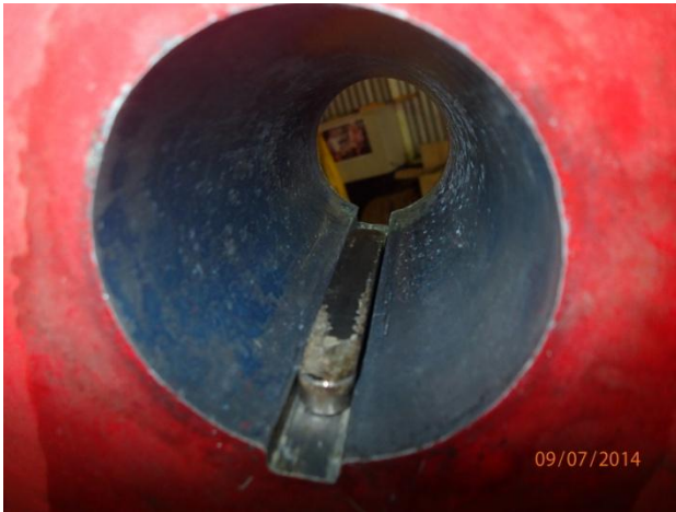
Key fitted in swing keel keyway
