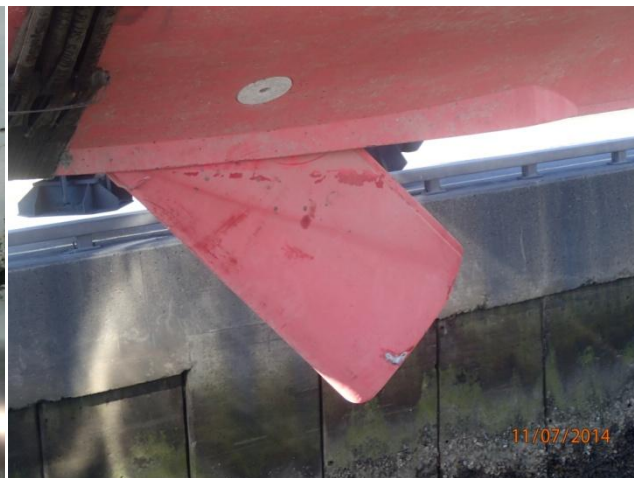
View of swing keel during retesting
