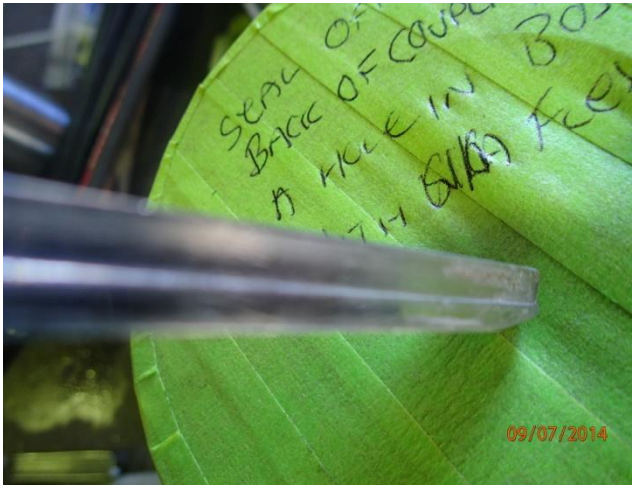
Key showing concave wear
