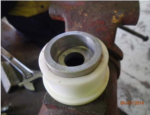
Port bearing spigot inside bearing
