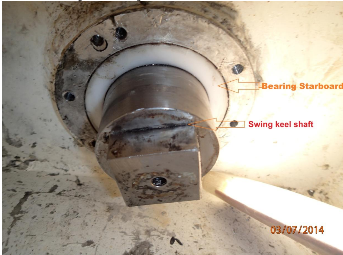
Starboard view of swing keel shaft arrangement
