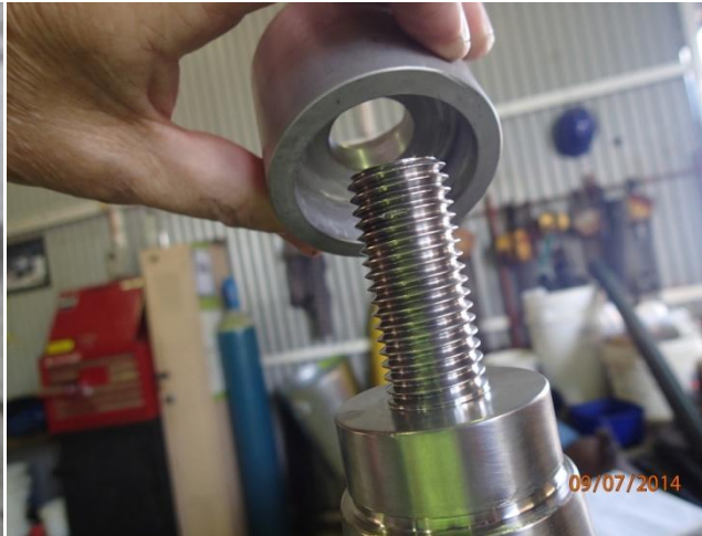
View of port side of shaft and bearing spigot
