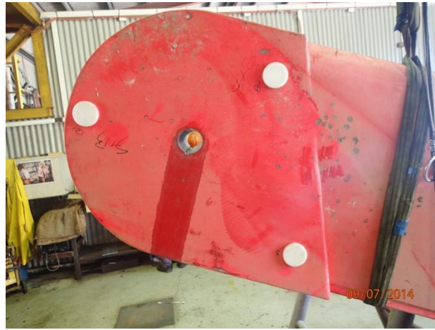
View of swing keel top with shaft housing central
