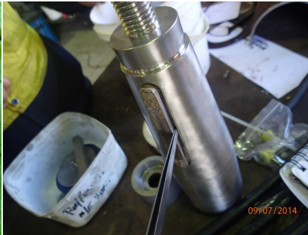
Clearance of key in keyway
