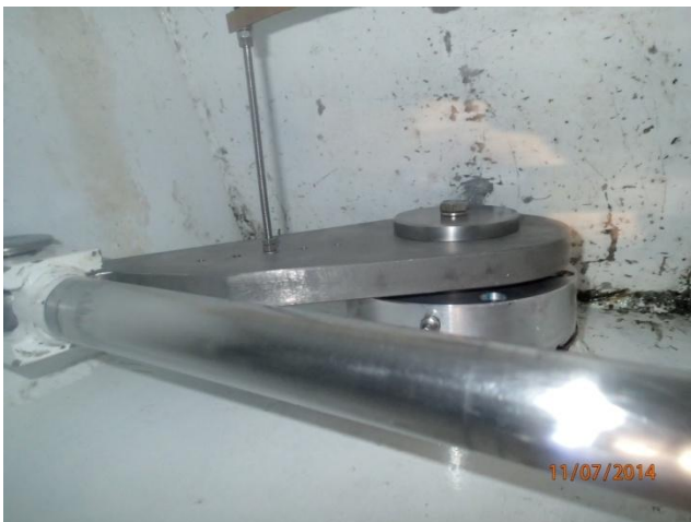
View of starboard side of assembled swing keel shaft and hydraulic ram
